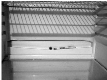
Don't forget to clean the "little hole" in the refrigerator.
